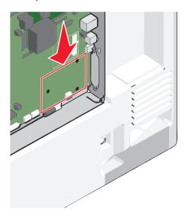
**4** Remove the printer hard disk.
